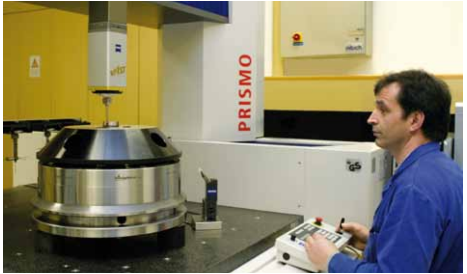
On the test bench is a Königsdorn® mandrel for the production of aircraft engines. The accuracy of the mandrel is checked and documented with a high-precision measuring machine.
