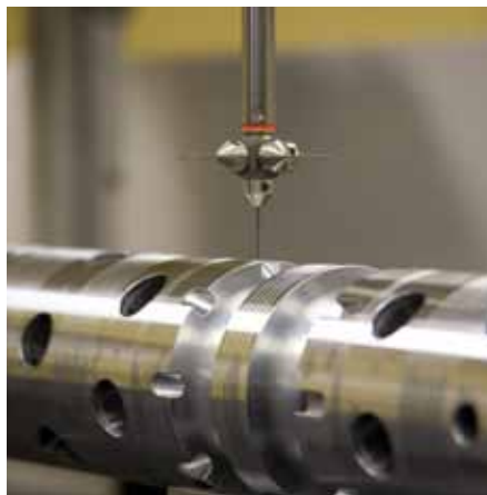
A precision measuring machine checks the accuracy of a hydraulic component with \mu (0.001 mm) precision.
